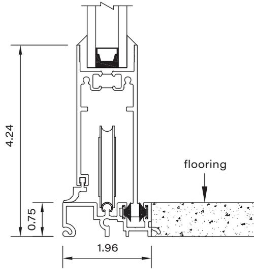
flush threshold with 1.81 diameter roller
